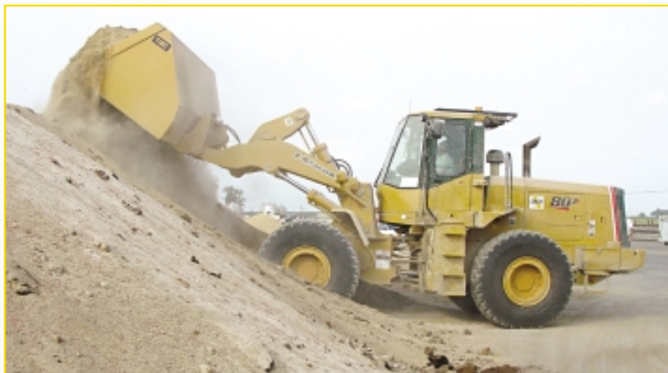
Kawasaki loaders run 24/7/365 and handle a wide variety of materials, much of it loose. Western Milling uses 5.5 cu. yd. rollout buckets on their 70ZIV-2, 7 cu. yd. on their 80ZV, 8.5 cu. yd. on their 85s, and a 10 cu. yd. on their 90s.
