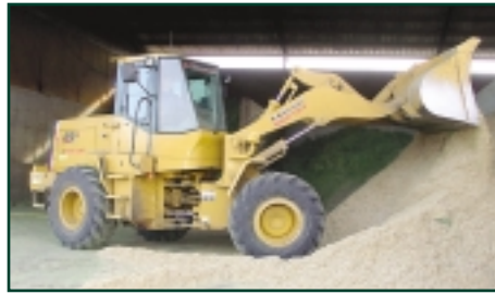
A 65ZV loader uses a wider, 70-sized bucket. It is not uncommon for dairies milking 3-4,000 cows to have six loaders. Dairies are also farms, growing hay and corn to supplement the specialized formulas they buy.
