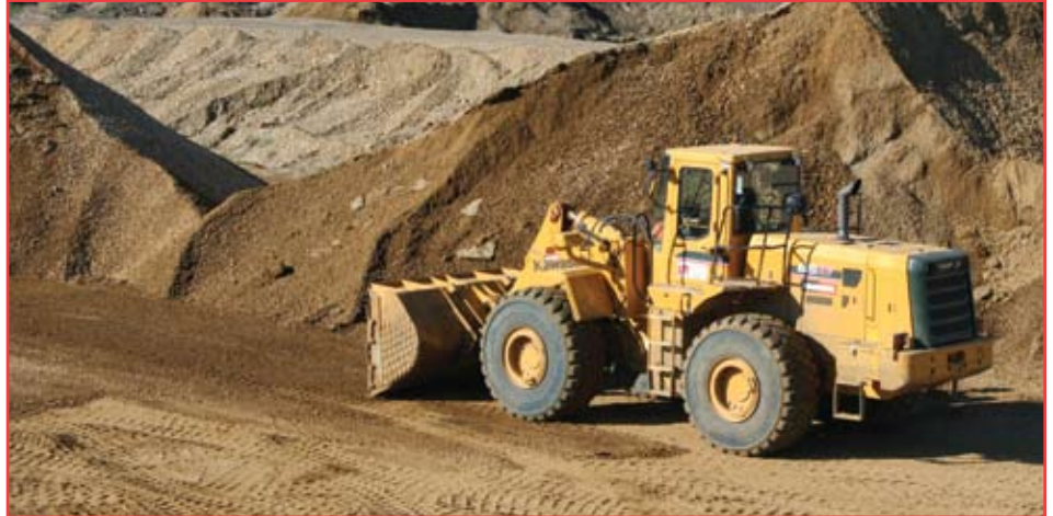
The well-balanced aspect of the Kawasaki loader, coupled with careful pad maintenance, eliminates rutting. Despite the abrasive nature of the material, the loader backdrams without resistance.
