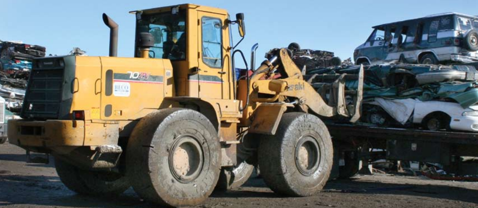
Metal Shredders equips their four Kawasaki wheel loaders with 60" forks, a quick coupler, and solid tires. Their 70ZV-2s also have autolube.
