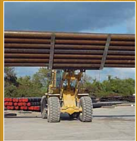
The company's 70ZV-2s use an extra counterweight and 96-inch forks.
