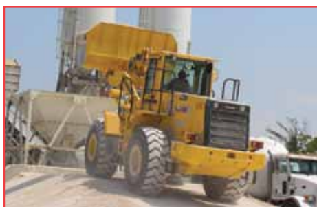
Kawasaki 80ZV-2 loader charges a hopper at the company's Lake Charles ready-mix plant. Note the white PAI concrete mixing trucks.
