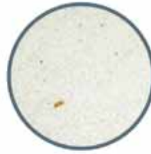
Target rating for hydraulic/transmission oils
