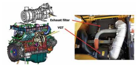
The DPF/Exhaust Filter is a rugged component that filters particulate emissions from the exhaust very efficiently. It replaces the muffler. The DPF is very effective in trapping particulate emissions. Passive and Active Regeneration keeps the DPF element cleaned without any action required by the operator.
