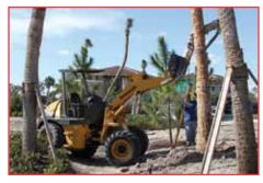
Those palm trees don't grow there by themselves. These stately accents must be planted. Kawasaki's oscillating axle maintains ground contact while in a swale. Frame-style oscillation helps maintain a more consistent lifting capacity.
