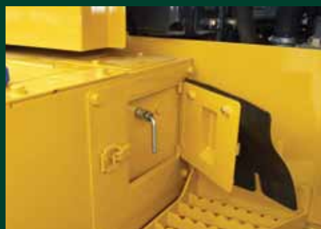
The Battery Disconnect Switch, standard on all Z7 models, is conveniently located at ground level.
