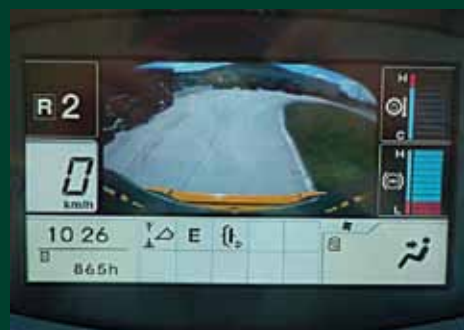
A Backup/Rearview Camera is crucial to safety. It's standard on all Z7 loaders introduced to date.
