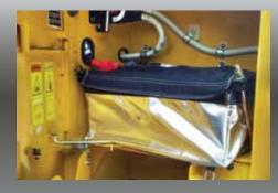
Batteries are isolated and insulated. The wiring harnesses for the chassis, transmission, and cabin are high-heat resistant.
