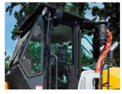
All-new cab-window design utilizes blast-resisting tempered glass that is then set in a reinforced retaining frame. E-Coat helps block external corrosives.
