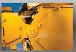
Belly guard provides protection for the front chassis and transmission.
