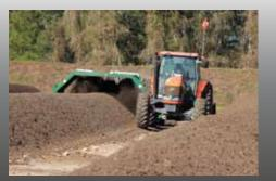
Compost rows are placed on a 4-inch clay base with 9 inches of lime rock on top that is then packed down to about 6 inches. The windrow turner typically takes 20 minutes to do a row, longer if water needs to be added.
