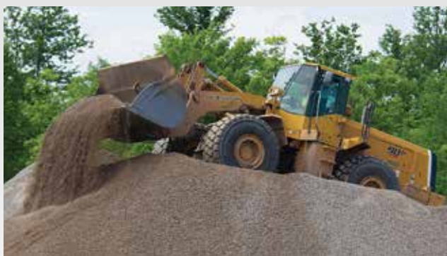
Smaller Kawasaki (KCM) loaders are used to load dump trucks and manage the piles of crushed material.
