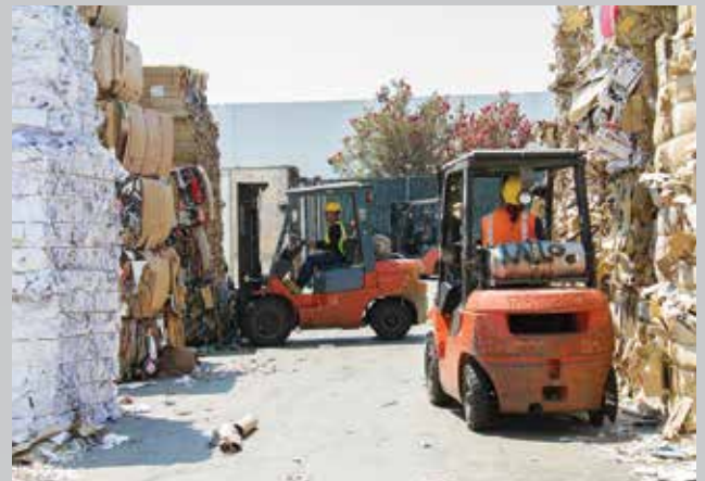
The waste paper and cardboard is sorted then baled for easy loading into containers.
